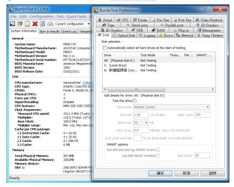
3.1.2 show Disk test mode(default cyclic -- 10 ways cycle test)
