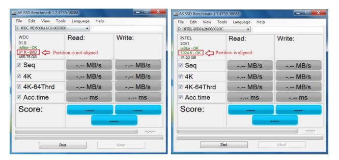
**XUsing AS SSD Benchmark to check vendor AHCI Drive is installed**
